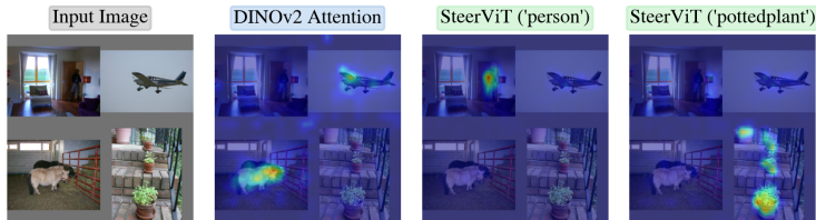
Fig. 6: Text enables targeted attention. Attention maps on a four-image mosaic demonstrate that text conditioning with SteerViT redirects self-attention to the queried concept whereas DINOv2 attends to the most prominent objects. Note that the [CLS] -token of SteerViT was not directly optimized for targeted attention and remains frozen in its original state.
